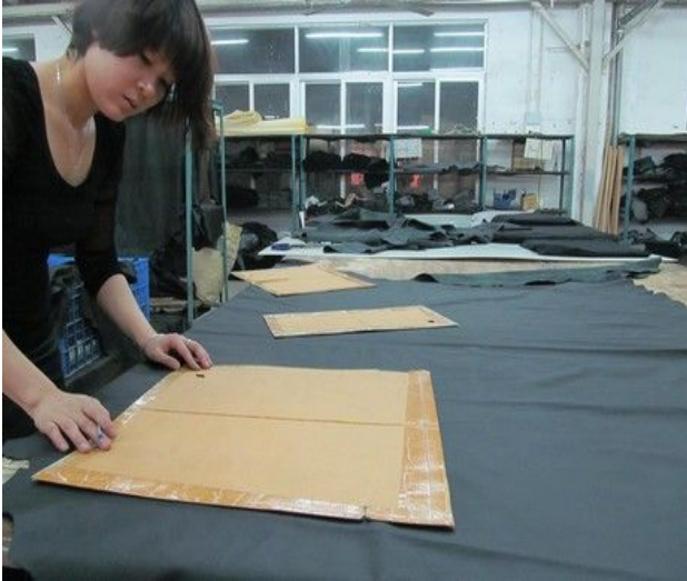
Cut fabric by moulds (剪布)
