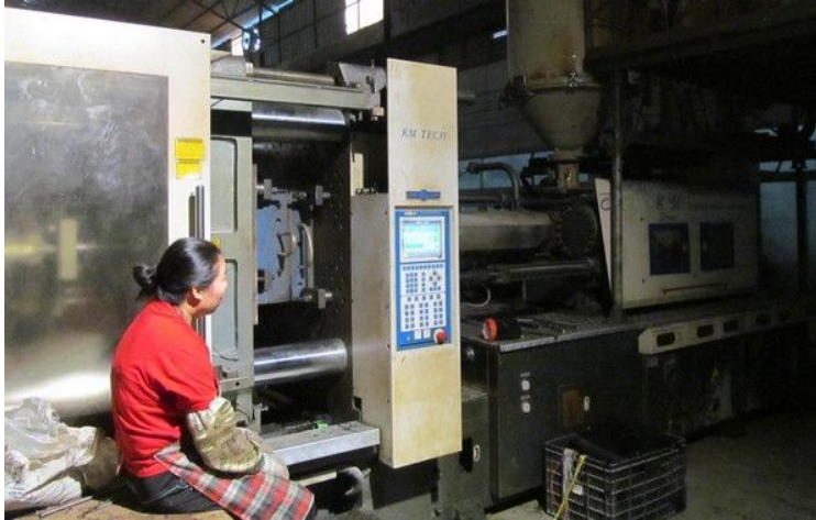
worker are operating injection machine 工人在操作注塑机
