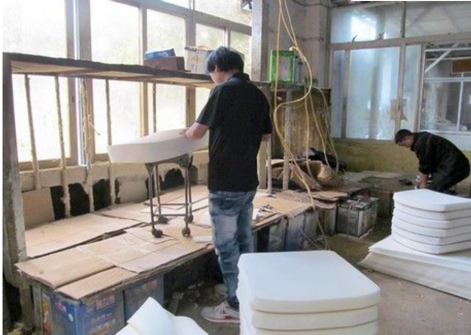
sticking foam on the board (在木板上粘海绵)
