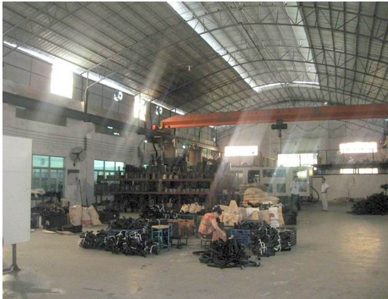
worker are cleaning the plastic components, cut burrs and pick up the defective parts. 工人在清洁塑料配件，切掉披锋 和 选出不良品
