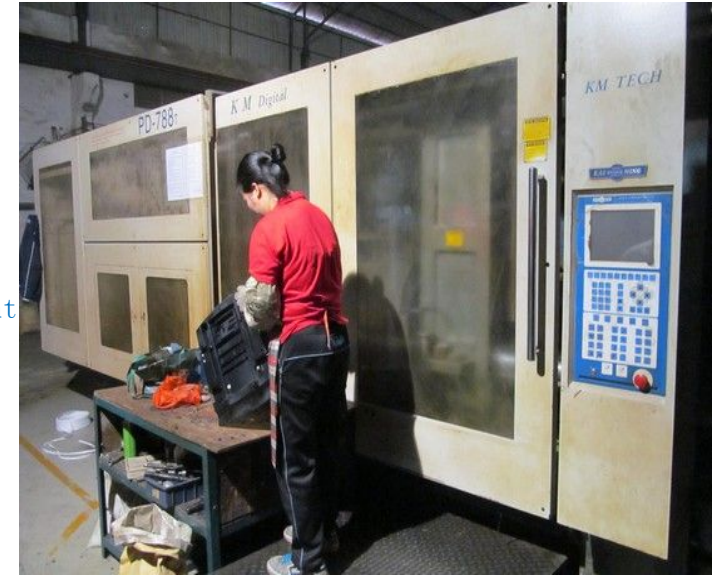
worker are cleaning the plastic components, cut burrs and pick up the defective parts. 工人在清洁塑料配件，切掉披锋 和 选出不良品
